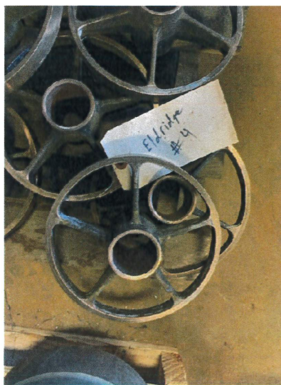
Column spiders with bearing inserts removed
