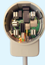
TRUSense Fiber Gateway: Connects directly to fiber by use of a Small Form-factor Pluggable (SFP) Optical Network Terminal (ONT)
