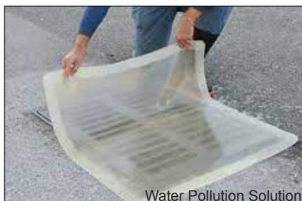
**Storm Drain Covers/Mat:** These are placed on the top of storm drain inlets to prevent washwater from entering the drain. They allow washwater to pond and be collected with a sump pump or shop vac.
