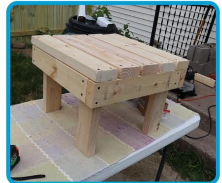
Measure across the frame from outside to outside (in this case it was 19.5"). Cut five boards and screw into the top of the frame.
